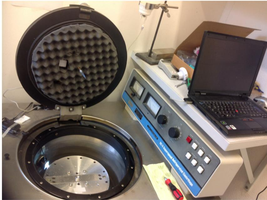
Figure 1- Cavatron with big rotor (diameter = 28 cm)
